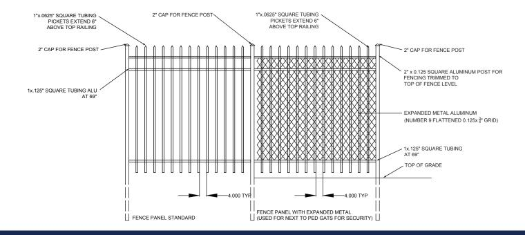
**ACT Fence Panels** are constructed from solid welded aluminum—no screws, no rivets—delivering a sleek, tamper-resistant solution built to last. Each panel measures 6 feet wide by 6 feet tall, and lengths can be easily trimmed on-site to fit smaller gaps or custom configurations. We keep plenty in stock and can quickly ship panels upon request, so your project stays on
