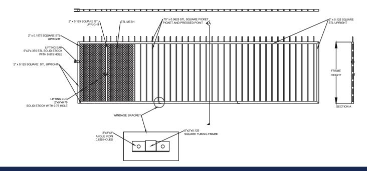
The **Vertical Lift Gate** is a popular style in the self-storage industry, mainly because it has the smallest footprint, taking up roughly a 7'x4' area on one side of the entrance. This gate style pivots up on its heel and out of the way, standing up over the operating unit itself. It is the fastest-opening gate style, meaning less waiting to enter a facility. Also, any size truck can be driven through the gate opening without worrying about the gate impeding the vehicle.
