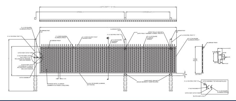
If you're looking for a durable, easy-to-maintain gate that slides open to allow access to a facility, the **ACT Cantilever Slide Gate** may be your answer. The cantilever gate is supported by rollers that keep the gate suspended above the ground, braced on each side by support posts, meaning it does not sit on a track and slide open and closed.
