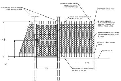
The ACT Pedestrian Gate is made from powder-coated steel for years of durable protection against rust and corrosion. It incorporates self-closing hinges for ease of use and offers added security with expanded metal welded directly to the pickets to help avoid unwanted entry from the outside.
